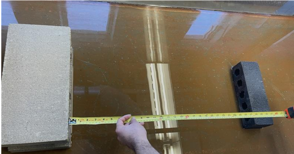
Figure 38 Placing bricks at different known locations for testing and ML training
